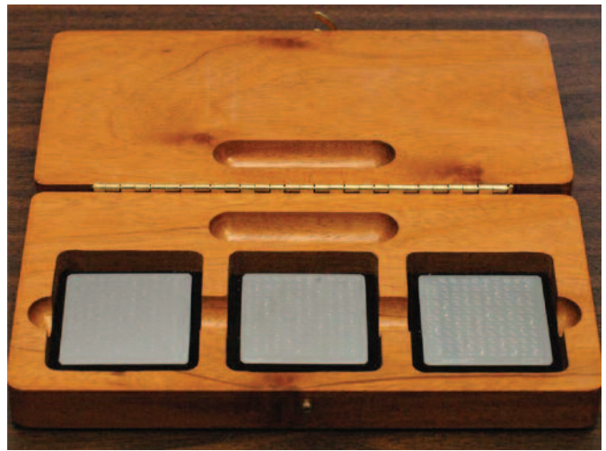
Figure 1. Photograph of PT artifacts for Rockwell hardness.
